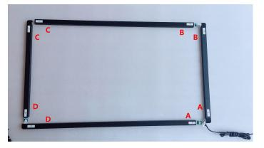
At the corner of AD, lift the black buckle up for the connector in the A side.(Please don't too hard, is damaged easily). Pick up the AB side, Insert the A-side FPC cable(blue face is up)into the AD side FPC connector, and lock the buckle. The FPC cable unfold ,easy to break. when connect well ,be careful to push the PCB into the frame. As showned photos:
