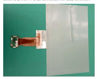
3. After connecting the touch foil FPC tail with controller, then pls connect USB controller with PC via USB cable, connecting method as below picture:
