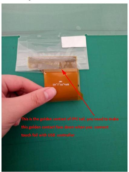
15inch to 24inch FPC tail connected with USB controller:
