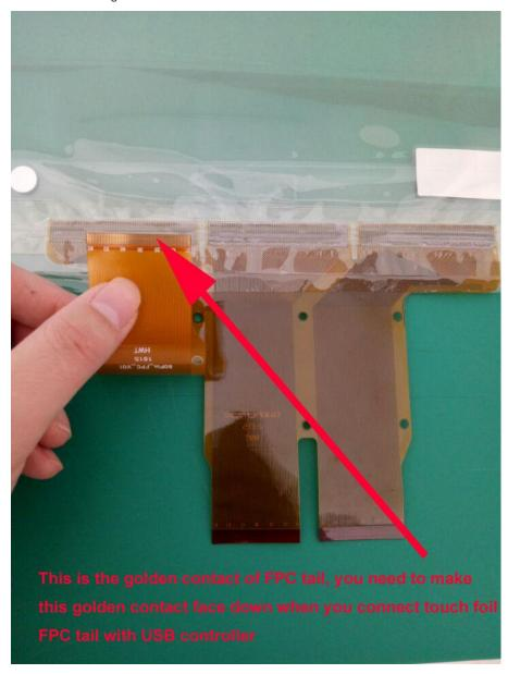
27inch to 84inch FPC tail connected with USB controller:
